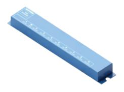
An interface that can receive signals from up to 8 RFID antennas, and communicate those signals back to the Outform network.
