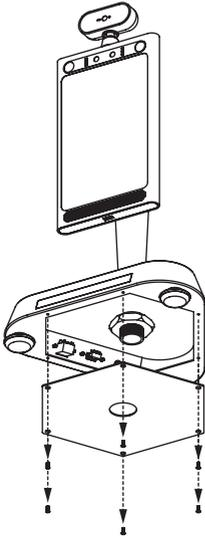
Step 6. Disconnect DC/RJ45 USB cable like the drawing shown below, and take out all the cables out from Counter base.
