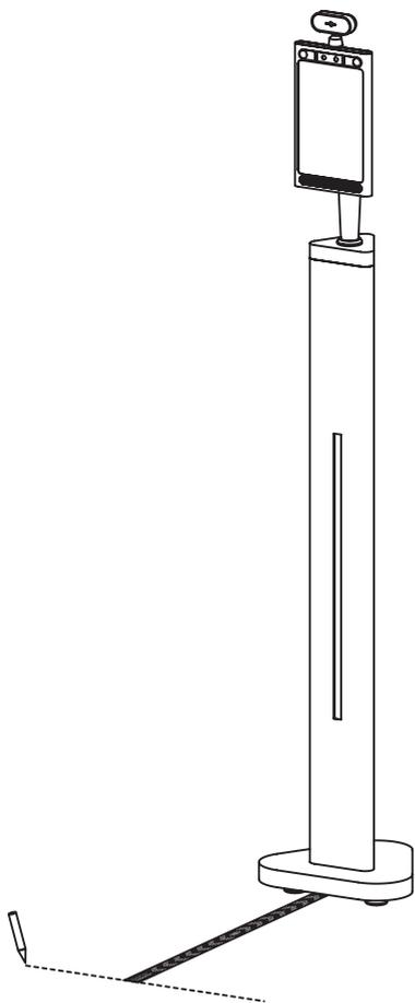
Step 4. Using the line drawn in step 3 as a guide, remove the protective film on the backside of the reflective sticker, and place the adhesive side on the floor.
