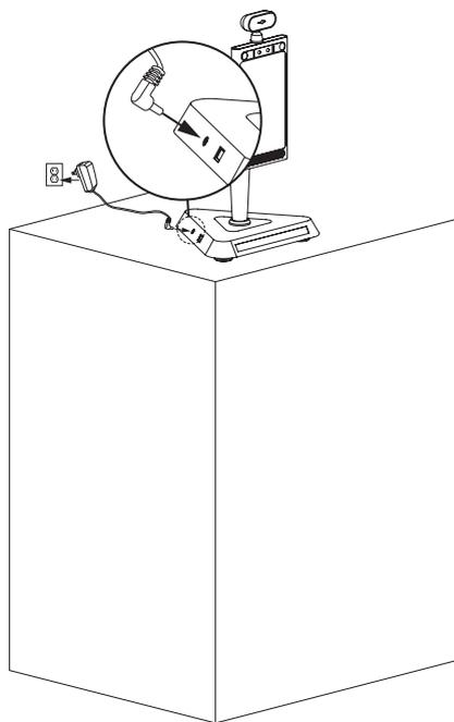
Step 4. Use the reflective sticker to measure the correct standing distance from the front of table, as pictured below. Use a pen to draw a straight line about 50 Centimeters (1.97 Inch).
