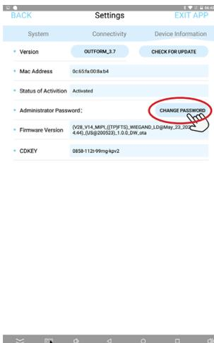
Step 4. Password page is showing. Enter a password in "New Password" input box and confirm again. Then click "OK" to save the password.
