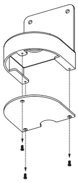
Step 4. Tight wall bracket with Self-tapping screws (x4) to the pre-installed expansion screws in step 2.
