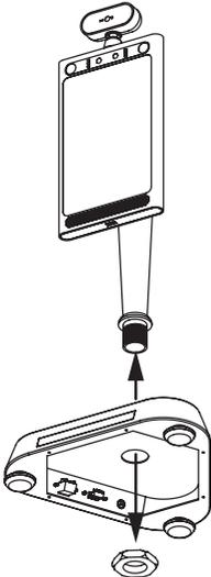
Step 8. Install Thermometer to pre-installed wall bracket by tight the big nut that removed from last step.
