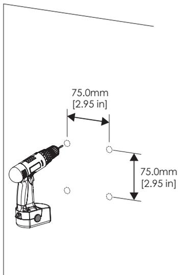
Step 2. Apply expansion screws (x4) to the wall.
