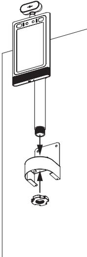
Step 4. Reinstall M3 screws (x3) that removed from step 3 to apply bracket bottom piece.
