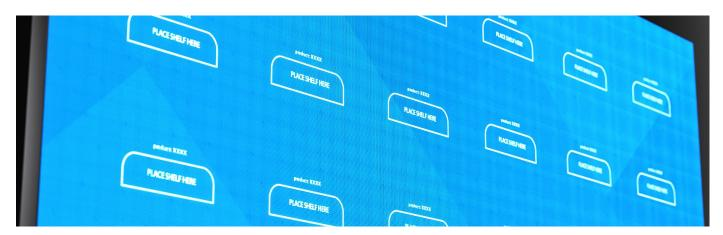
**PROTECTION** A protective film on the face of the LED is used to provide durability for the panels. Made of a sealing spray, the protective film encases the LEDs without affecting the refracting index, light transmission or brightness loss. The film also adds anti-collision, anti-shock, anti-UV, water proofing, dust resistance, and heat dissipation that extends the life span.
